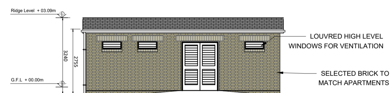
BLOCK L BIN STORE - SOUTH ELEVATION
